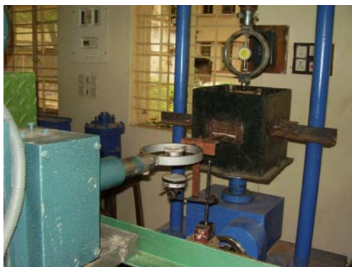
Figure: Field Pull-out testing unit for Reinforced Earth Technology
