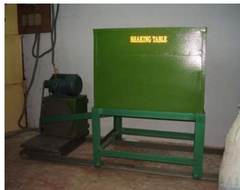
Figure: Shaking Table for testing Model Reinforced Earth wall
